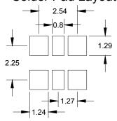
Note: LVDS VCXOs are designed to fit on Industry standard, 6 pad, layouts.
